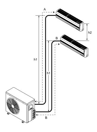
CAUTION: Capacity is based on standard length and maximum allowance length is on the basis of reliability.
